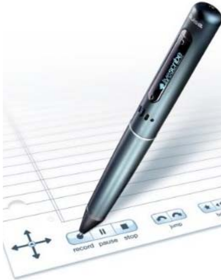
Figure 4: The pen interacting with the digital paper interface. It is currently poised on the record action which will allow it to record the audio information in sync with written notes.
