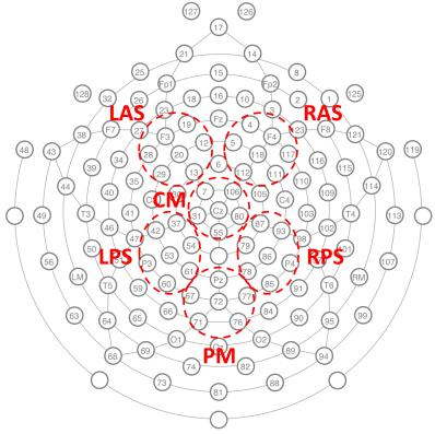
Fig. 3. The 128-channel GSN electrode locations used to record the EEG and the six channel groups where classification analysis was conducted. LAS: left anterior superior, RAS: right anterior superior, CM: central medial, LPS: left posterior superior, RPS: right posterior superior, and PM: posterior medial.
