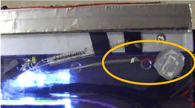
Figure 3: Piezoelectric sensor attached to the surface
